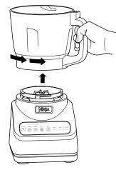
**8** To remove the bowl from the motor base, turn the bowl anti-clockwise and then lift it.
