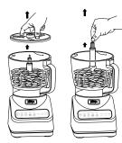
8 Using the finger holes, carefully lift the disc out of the bowl. Then, grasp the adapter by the top of the shaft and lift it out of the bowl.
