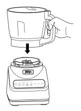
**2** Lower the Food Processor Bowl onto the motor base and rotate clockwise until it clicks into place.
