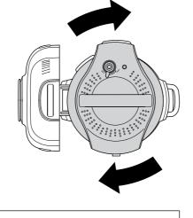
NOTE: The pressure lid will not unlock until the unit is completely depressurised.
