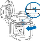
Install Pressure Lid by aligning the arrows on the lid and base, then turning clockwise until lid clicks into place.
